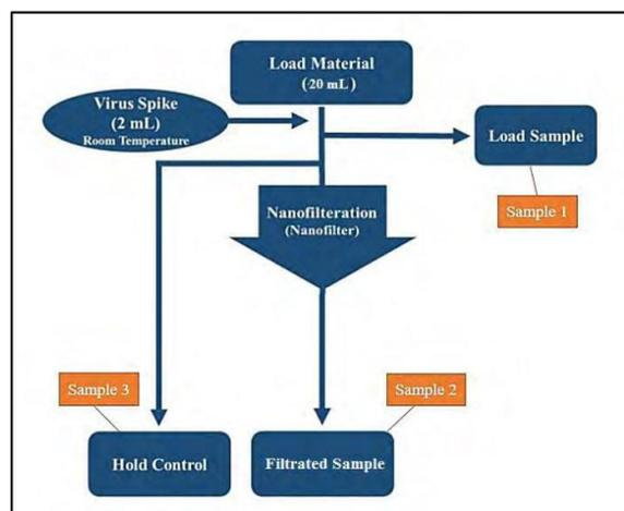
Fig. 4. Nano Viral-filtration step; procedure and sample
