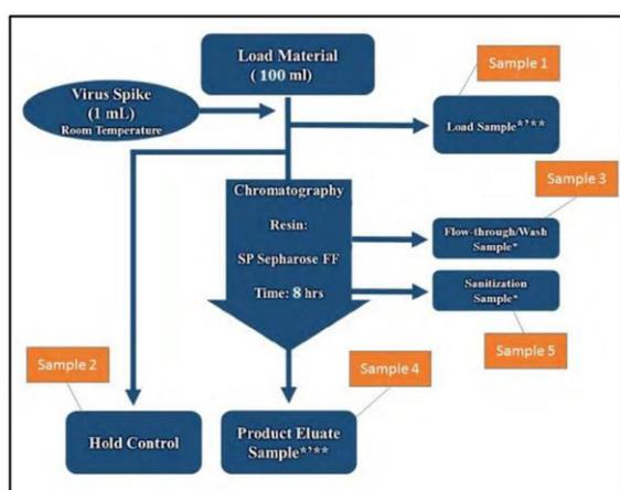
Fig. 1. Cation exchange chromatography step; procedure and sample
