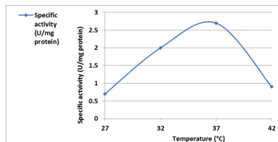
**Figure 3.** Effect of temperature on the specific activity of L-Met enzyme
